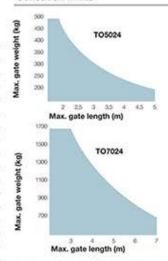
The shape, the height of the gate and the weather conditions can considerably reduce the values shown in the graph to the side.
